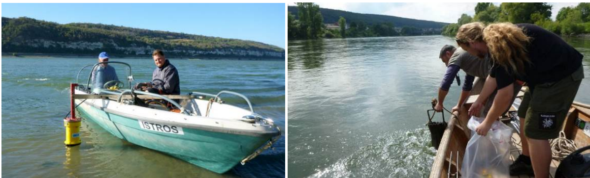
Figure 1: Discharge & velocity measurements (ADCP) Figure 2: Bed material sampling (bottom sampler)
