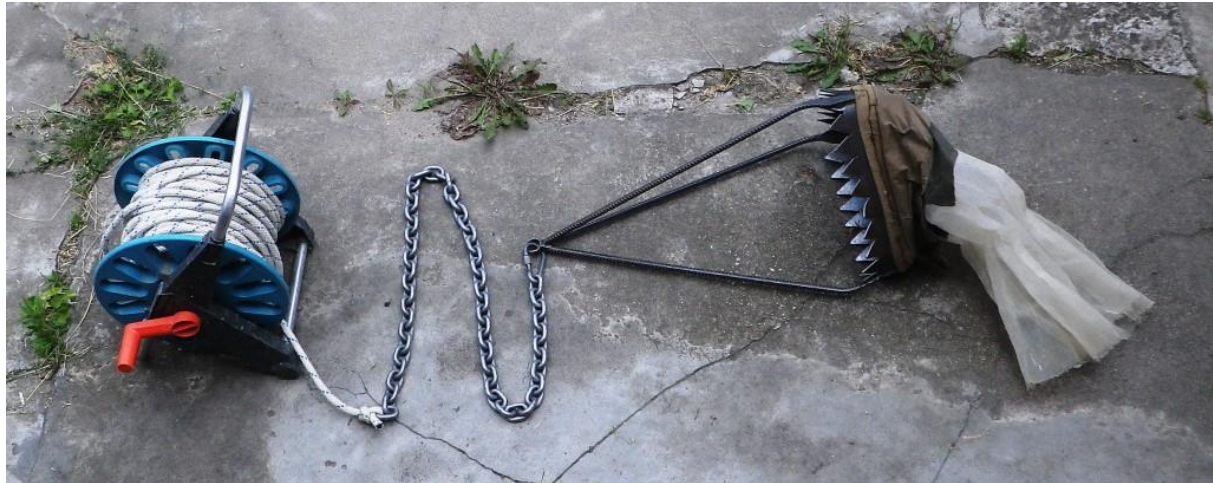
Figure 51: Bottom dredge with chain and rope for macroinvertebrate sampling
