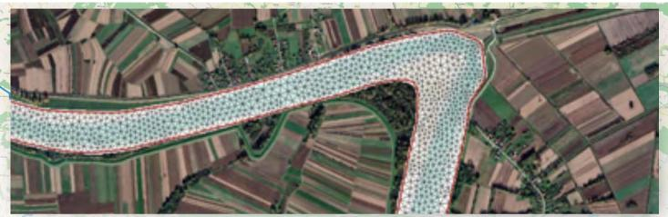
Figure 1: An example of a model mesh with the underlying terrain grid
